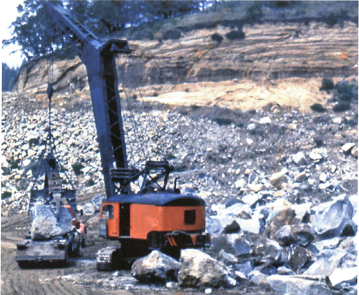
Figure 6. Sorting & loading "A1" stone, 15 tons. Note: 20 ton Semi truck.
