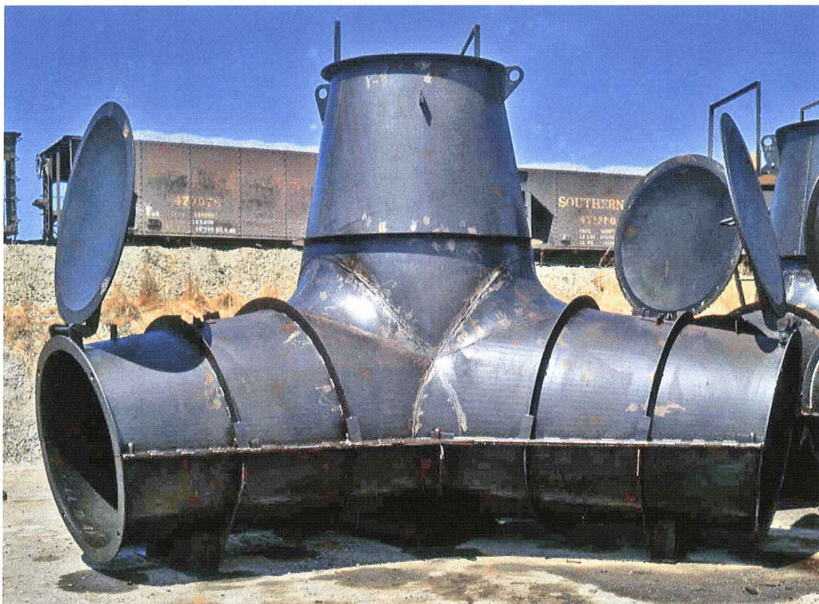
Figure 30. Sheet metal tetrapod forms. One of eight tetrapod forms.
