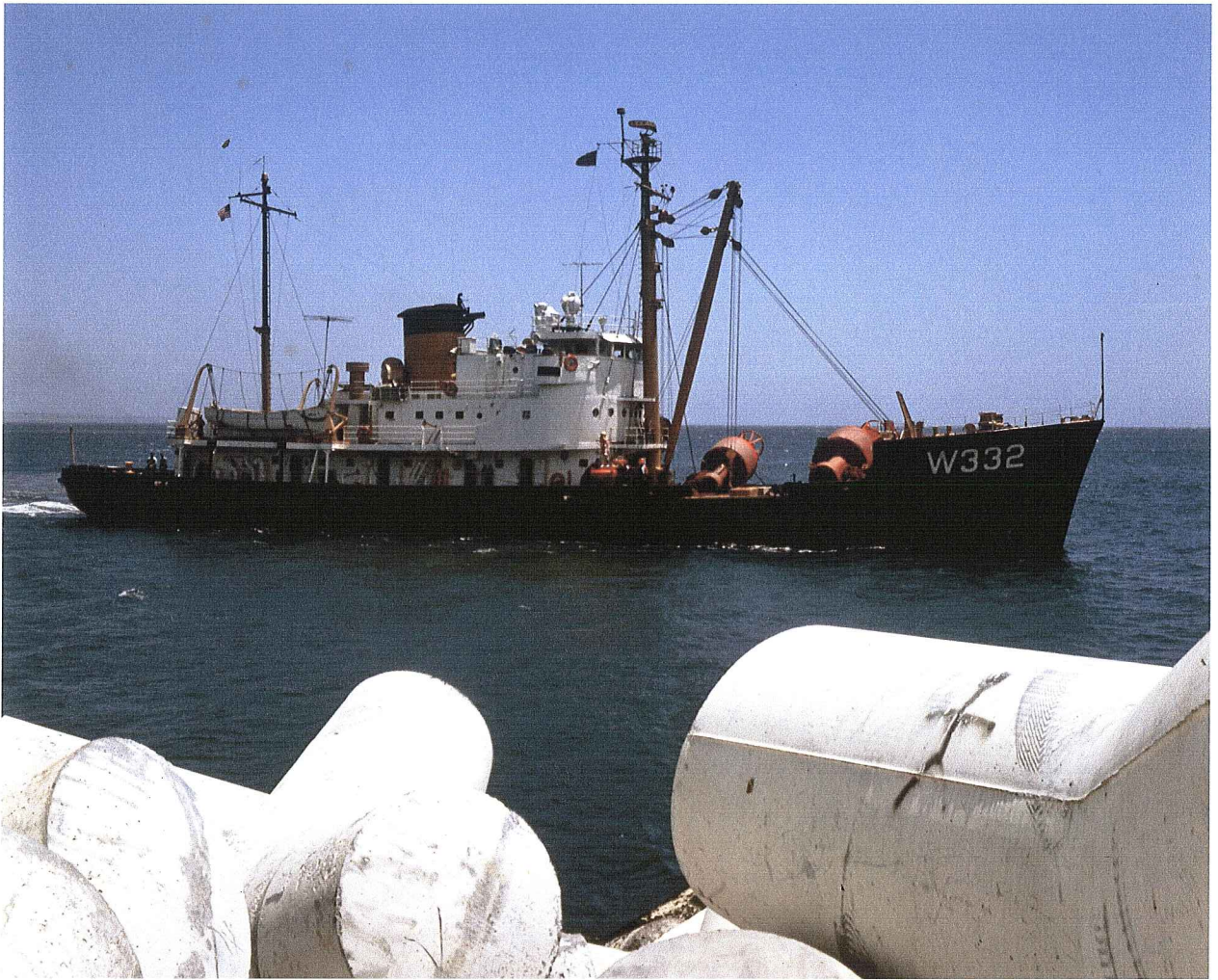
Fig. No. 11. Coast guard boat laying the buoys to outline the channel.
